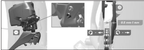
Fig. 97 Setting the upper stop ©Sram
